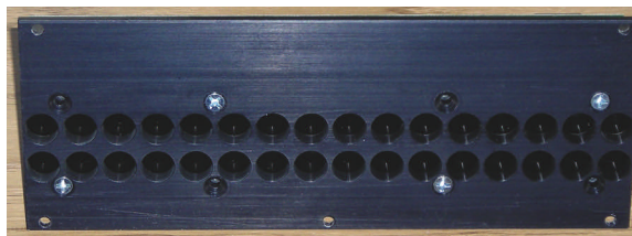
FIGURE 3. A test fixture contains holes that pass light between 32 sensors and a test board.
