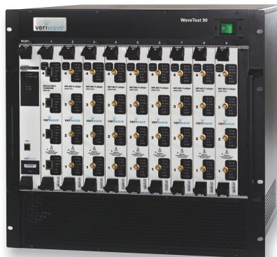
During the LACMA wireless LAN prequalification testing, the VeriWave WaveTest 90 and WiMix test suite provided load and client capacity tests.
